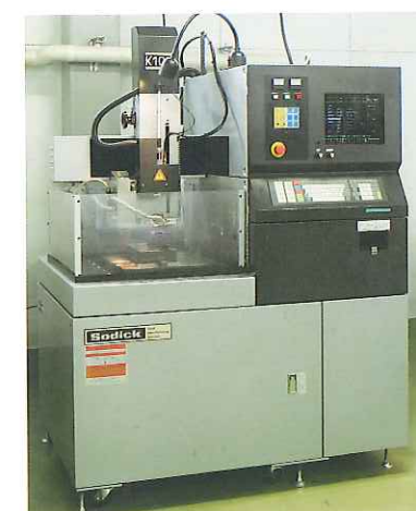
NC高速細穴放電加工機 NC high-speed small hole electric discharge machine
